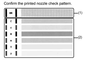
(1) If lines of this pattern are missing, the print head nozzle needs cleaning. Example: When lines are missing (Black ink)
